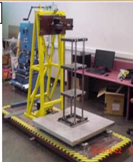
Figure 1 Uni-axial earthquake simulator (shake table) for earthquake engineering research and education
