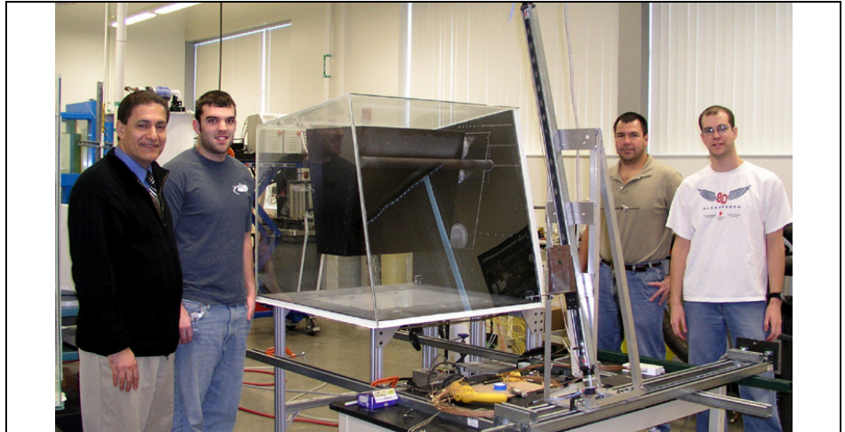
Some of those involved in the engine heat research are (from left) Dr. Parviz Merati , MAE chair and project leader, Rob Messner , ME senior; Dr. Javier Montefort , MAE assistant professor; and Kevin Kalchik , ME senior. They are posing with a full-scale model of a car's engine block and exhaust pipes that was enclosed in a tempered-glass case to study the heat flow. Missing from photo are seniors Charles Gauthier (ME) and Thomas Spencer (AE)
