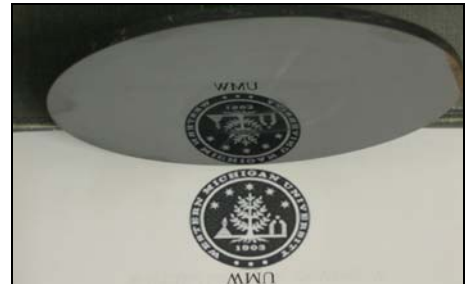
Figure 10: Picture showing the optical quality of surface finish on the machined CVD SiC sample
