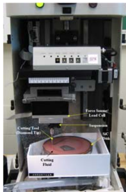
Figure 1: Machining Setup for the 6" CVD coated SiC disk
