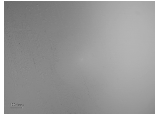
Figure 7(b): Image at 1000x magnification showing very light feed marks on the machined region (left side of image) after pass 2.
