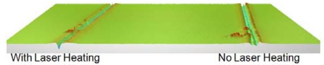
Fig. 7: 3D scratch profiles of the scratches with and without laser heating.
