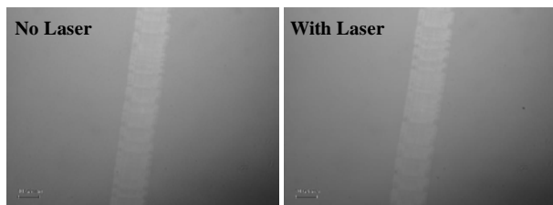
Figure 11: Region of the Si scratches, with and without laser heating, done with a 20mN (2g) thrust force.
