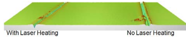
Figure 8: 3D scratch profiles of the Si scratches with and without laser heating (related to the same area imaged in Figure 7).
