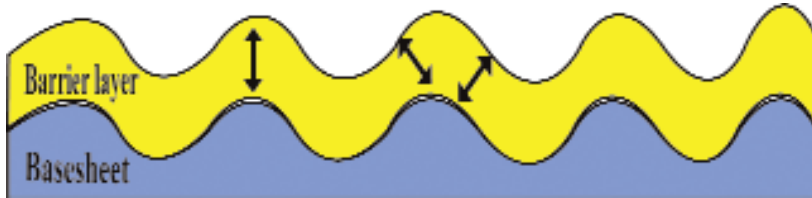
Figure 6. Thickness profile of contour coater
