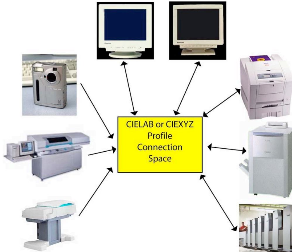
Figure 6. Open Color Management System with central Profile Connection Space (PCS).
