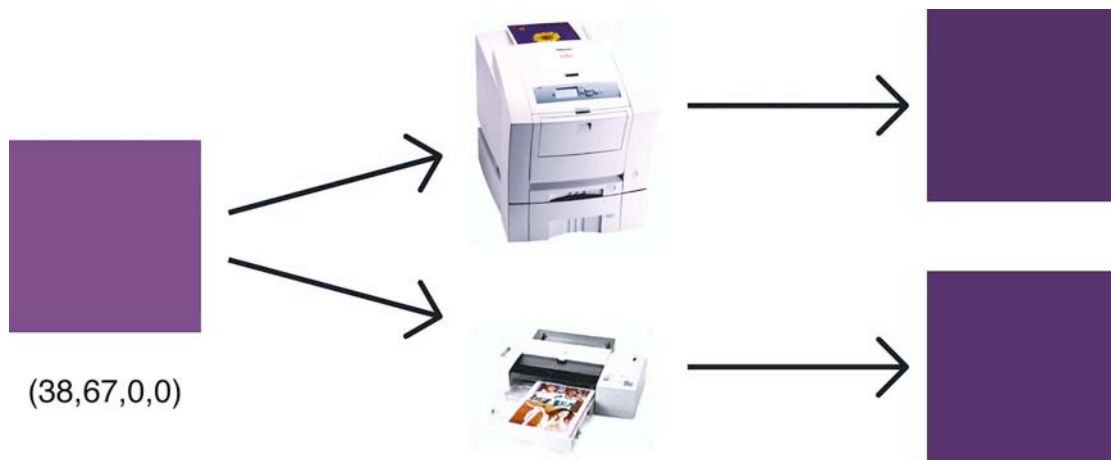
Figure 3. The same CMYK value printed on different printers will look different.
