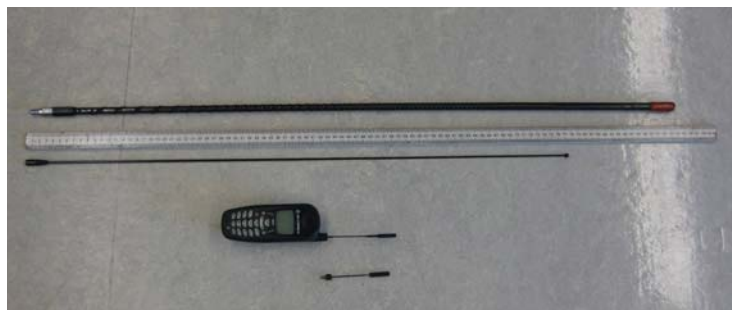
Figure 2: Antennas from three radio devices: CB (top), FM Car Radio (middle), Cell Phone (bottom).
