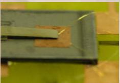
Silicon based Micro pressure sensor
