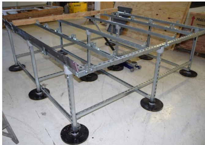
Figure 13: Shear Wall construction jig
