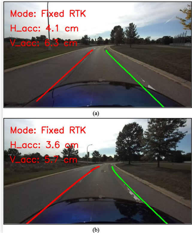
FIGURE 18 Campus Drive camera frame from a curved road segment with high-definition map lane line data overlaid on artificially occluded lane lines. Deviation from true lane lines occurs in this curved road segment due to the insufficient sampling rate of the GNSS heading sensor.
