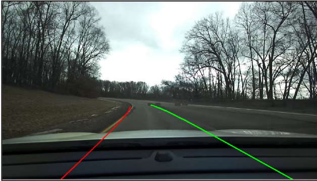
FIGURE 16 Eaton Proving Grounds camera frame from a curved road segment with high-definition map lane line data overlaid on artificially occluded lane lines. Deviation from true lane lines occurs in this curved road segment due to the GNSS operating in lower-precision RTK float mode and the insufficient sampling rate of the GNSS heading sensor.
