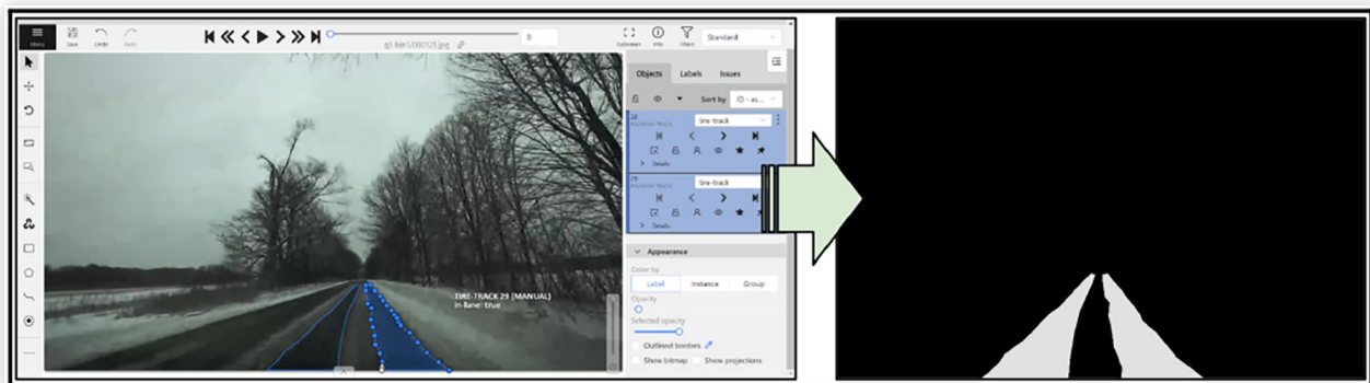
FIGURE 4 Example usage of CVAT for annotating the tire tracks with polygons (left) and the output mask of the labeling process (right).
