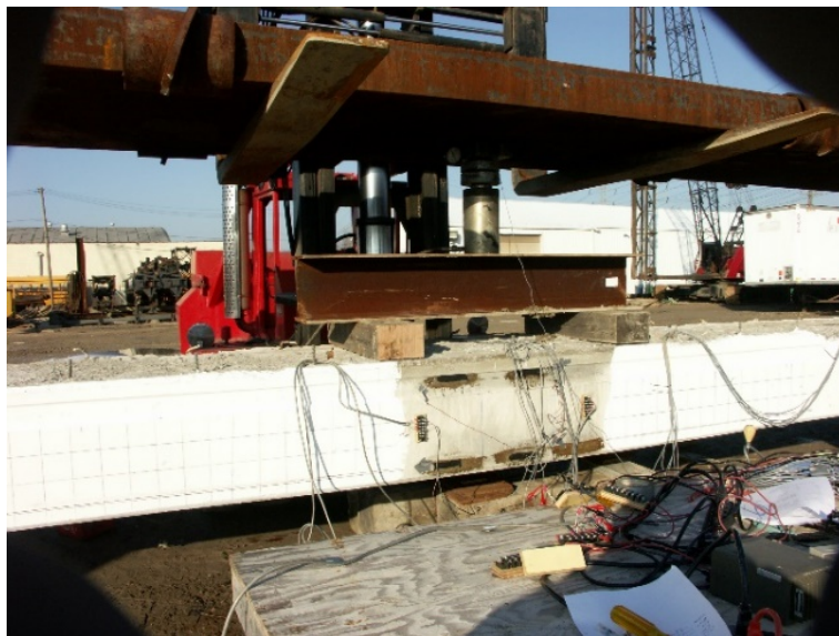
Figure 2-14. Load test setup for four-point bending test
