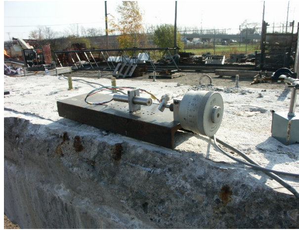
(b) Calibration of a DCDT at the site
