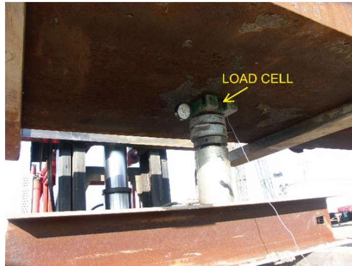
Figure 2-15. A closeup view of the hydraulic ram and load cell
