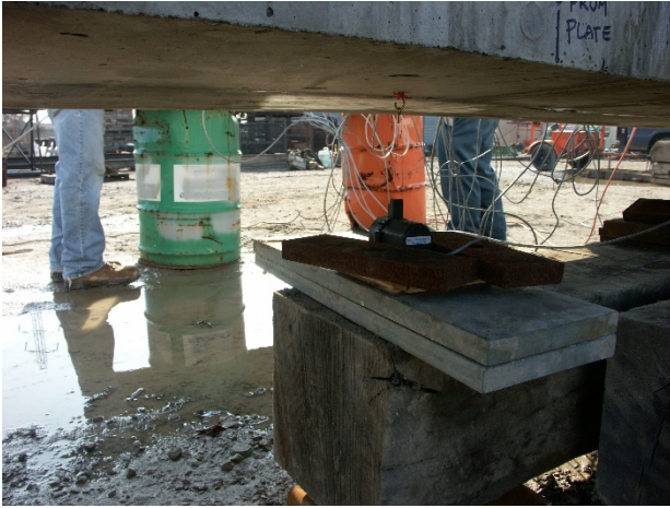
(a) CAPS setup for beam deflection measurement
