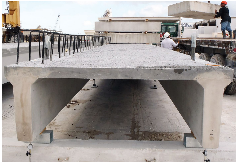
Figure 2-10. Load testing of a double tee beam at the fabricator's yard (Spadea et al. 2018)
