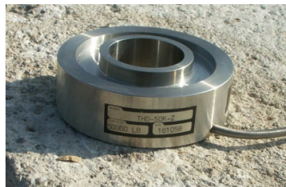
Figure 2-16. A closeup view of the load cell
