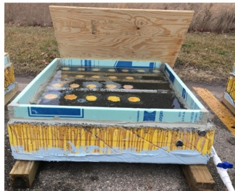
Figure 3-4. Slabs in the open parking lot and getting exposed to southwest Michigan weather
