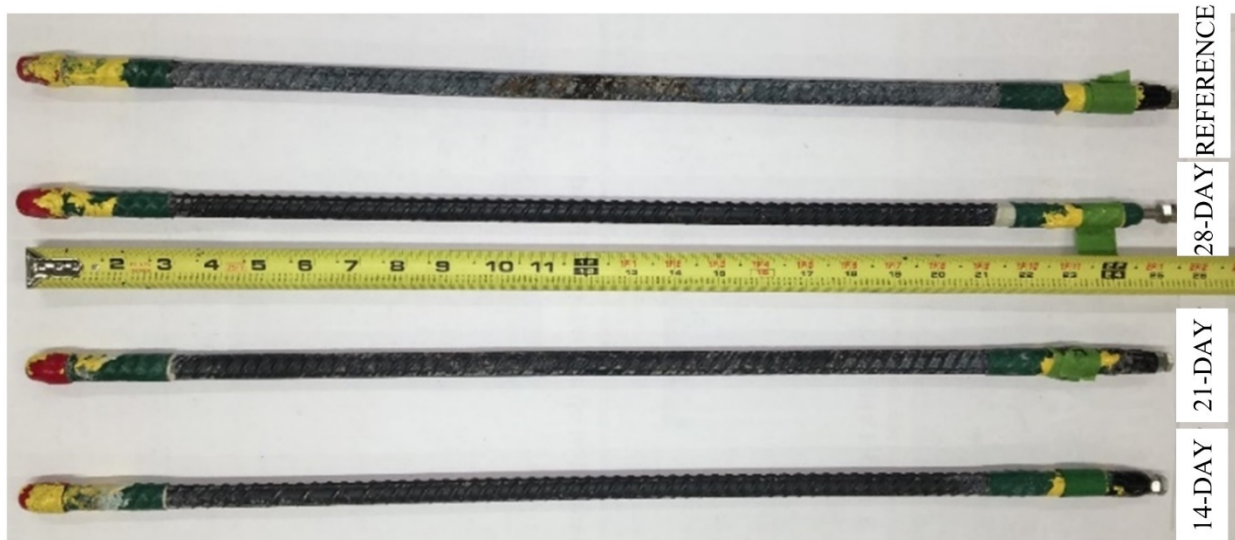
b) Reinforcing steel of reference and treated specimens
