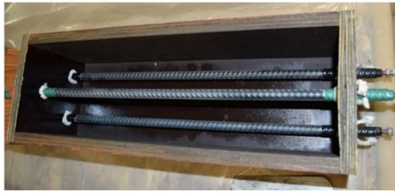
a) Rebar arrangement in the mold
