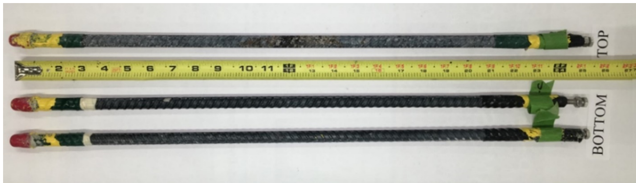
a) Reinforcing steel of a reference specimen
