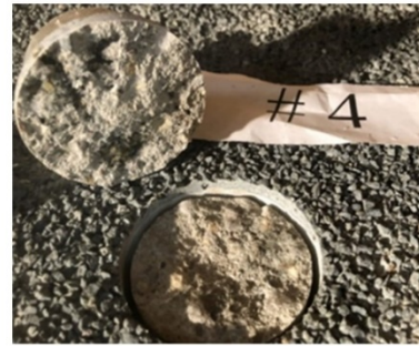
iv) Failure at room temperature following a heat cycle
