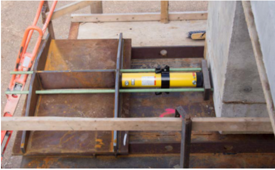
(a) Hydraulic cylinder with only pushing capabilities (Lesch 2015)
