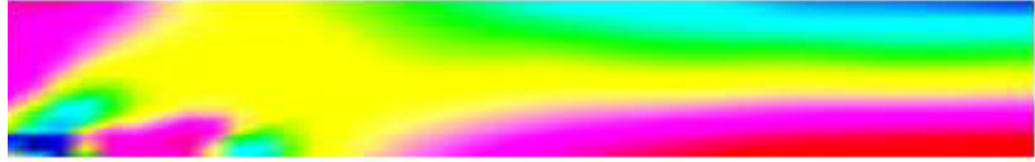
Axial stress trajectory of full length of box-beam (partial view, supported on left)
