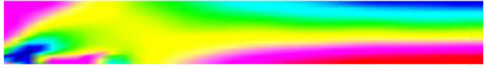
Axial stress trajectory of full length of box-beam (partial view, supported on left)
