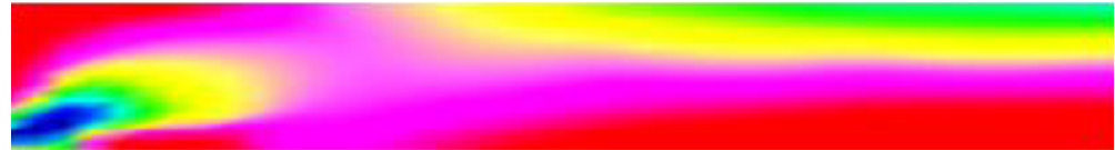
Axial stress trajectory of full length of box-beam (partial view, supported on left)
