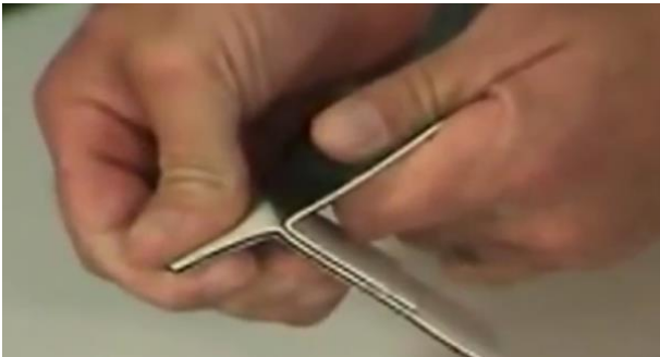
(c) Test cuts – Peeling off at the seams (IBRoofSystems1978 2012)
