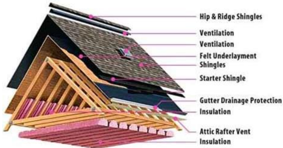
Figure 2-3. A typical steep sloped roof assembly (OldProRoofing 2014)
