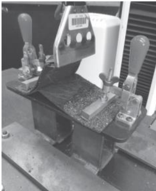
ASTM D6381 test procedure using Instron 3367 UTM (Dixon et al. 2014)
