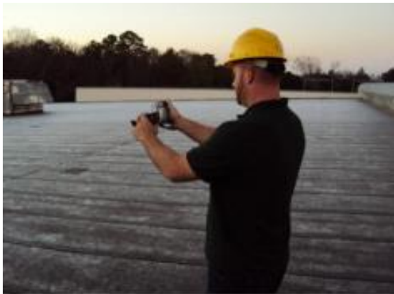
(a) Use of a handheld IR camera for roof inspection (Mullen n.d.)
