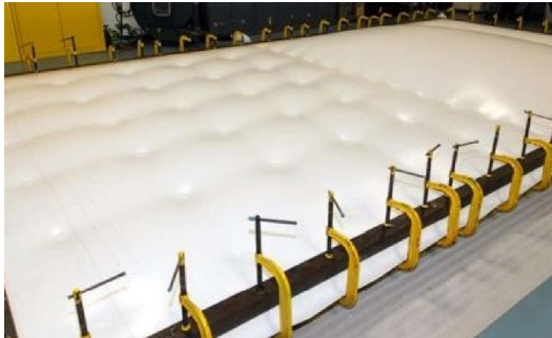
Figure 2-28. Testing of a Sika Sarnafil Rhinobond roof using a 12 ft × 24 ft frame (Sika n.d.)
