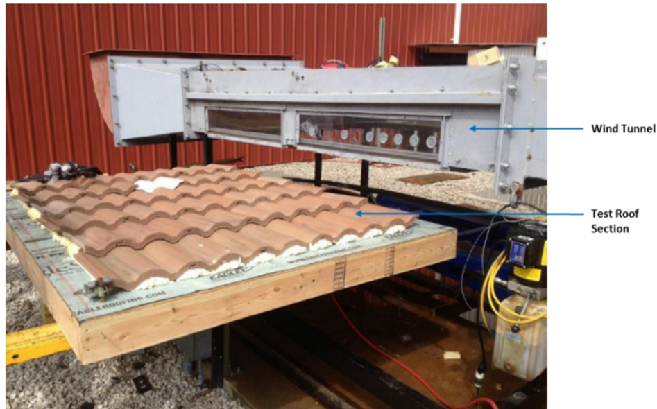
Figure 2-45. A specimen with roof tiles used in wind tunnel testing (Smith 2014)
