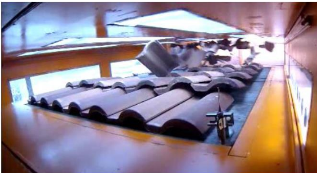
Figure 2-46. Failure of a specimen with roof tiles (Smith 2014)
