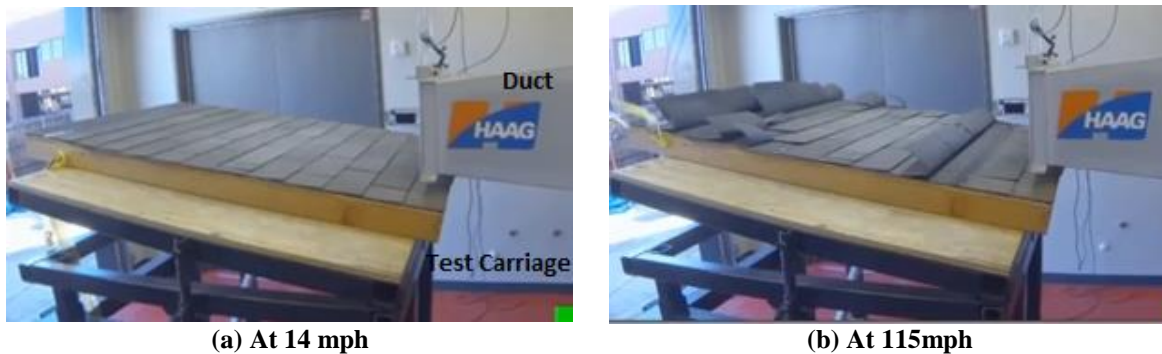
Figure 2-39. Behavior of composite shingles under different wind speeds (Haag Engineering 2015)
