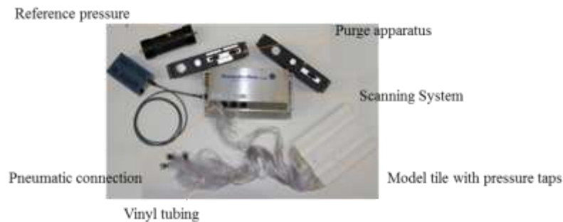
Figure 2-58. Pressure scanner (scanning system) connected to a model tile (Masters and Gurley 2011)
