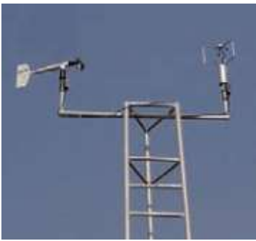
(a) 10 m tower and the location of anemometers
