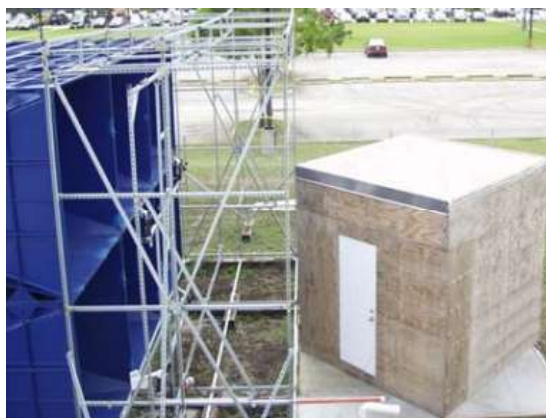
Figure 2-31. A test structure placed in front of the WOW at a 45° wind direction (Chowdhury and Blessing 2007)
