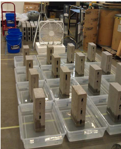
Figure 2. Masonry blocks in water
