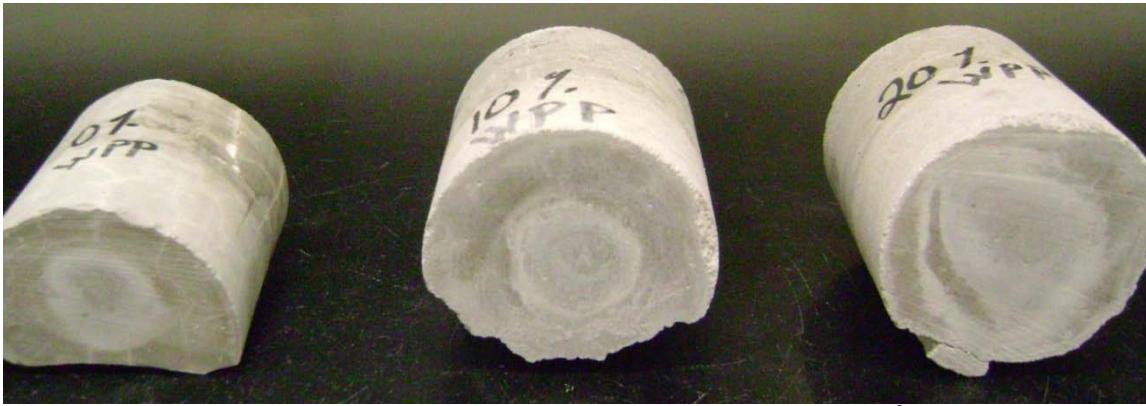
Figure 16. Specimens at the end of leaching test at 24 th day
