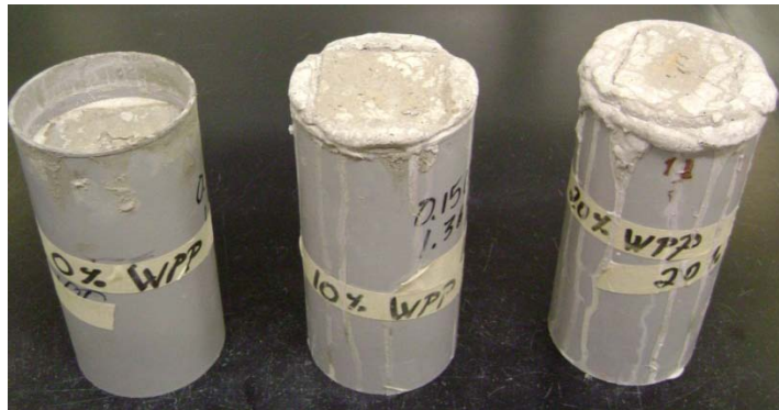
Figure 24. Specimens with 0%, 10%, and 20% WPP mix
