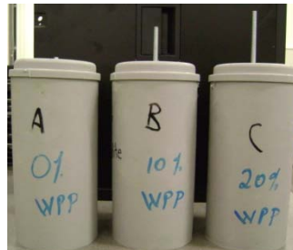
Figure 21. Piston tip elevation of 0%, 10% and 20% WPP mix after 1 day
