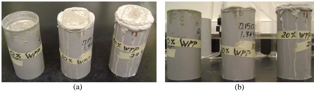
Figure 17. View of unusual expansion of cement grout with WPP
