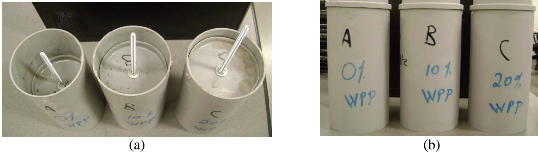
Figure 18. View of (a) cylindrical containers with plastic lids acting as pistons and (b) cylindrical containers with lids to guide the vertical movement of the piston
