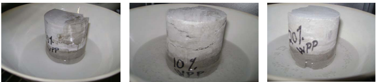
Figure 15. Specimens after 16 days (a) 0% WPP, (b) 10% WPP, and (c) 20% WPP
