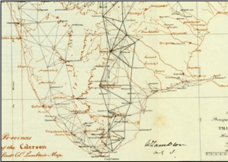
Figure 7. Southern tip of India from Kanyakumari northward to Dindigul showing triangulations of Col. Wm. Lambton of the Great Trigonometric Survey -- with secondary triangulations of others. Into these local surveys were "snapped". Arcot was 9 miles closer to "Madras" (Chennai) than previously thought. Triangulation error at Bengaluru (Bangalore) was thought to be only 7 inches!
