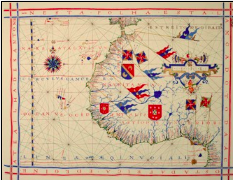
Figure 8. A portolan-like chart of the 17th century. Compass directions are given clearly over the Atlantic Ocean, with greater detail for coastal areas than inland. Whether this chart was based on a map projection, as we understand them today, is unknown.
