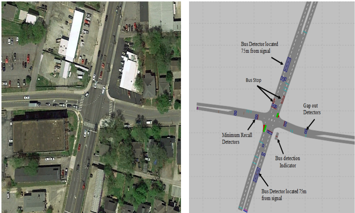
Figure 5: Sample of Study Intersection alongside its Corresponding VISSIM Model
