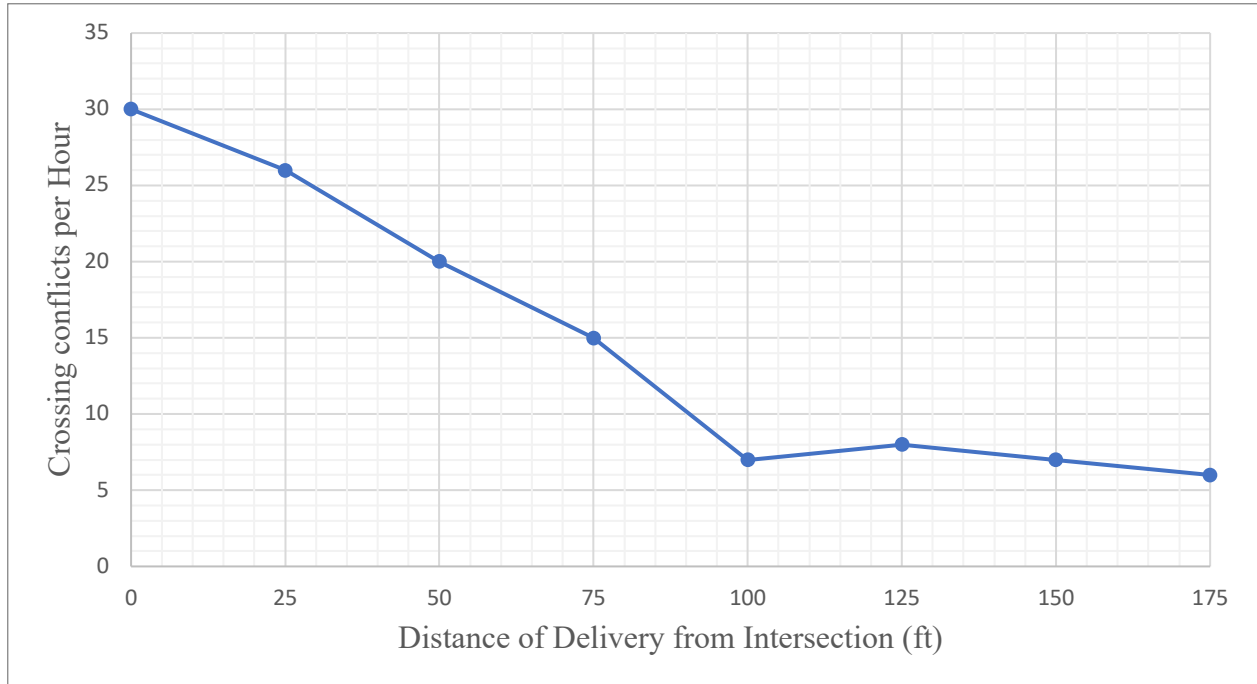
Figure 0.9. Effects of a bus curb stop location on the number of crossing conflicts
