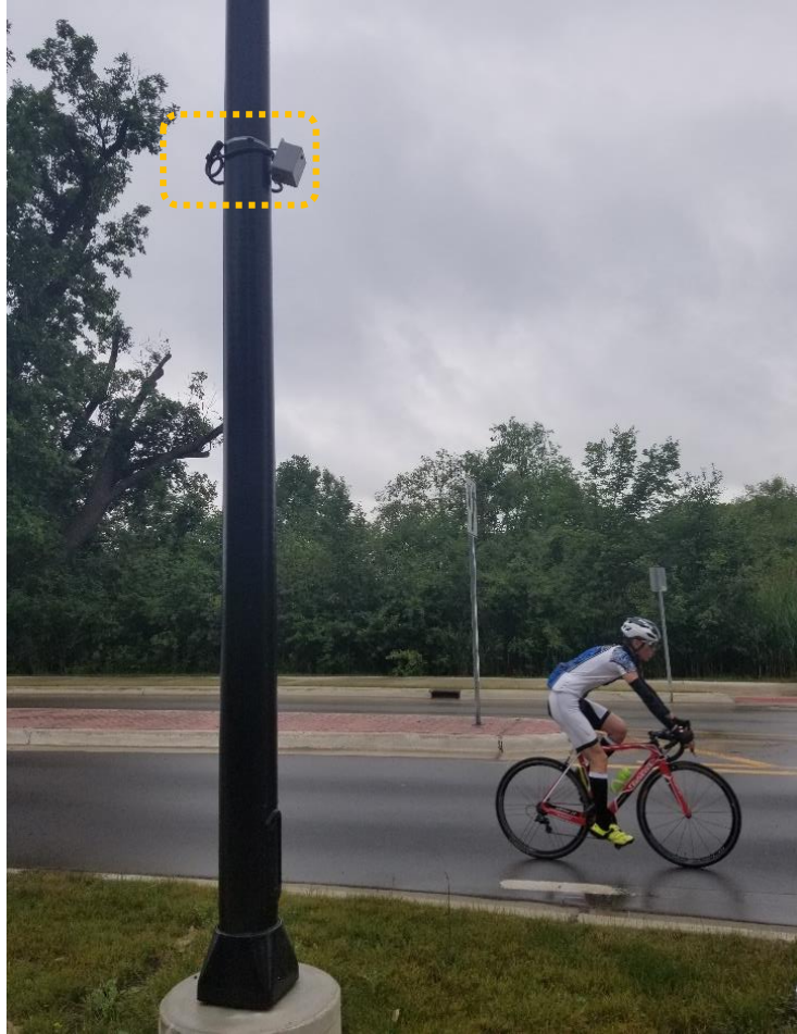
Figure 3.5: Position of the camera relative to the flow of cyclist in Nixon Road, Ann Arbor
